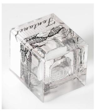
DuPont<sup>TM</sup> Surlyn<sup>®</sup> is used for a new decoration technology developed by DuPont and Oriol & Fontanel that allows to encapsulate textile fabrics such as lace for stunning effects.
