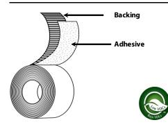
**Backing:** Printed Polyethylene Coated Cloth
