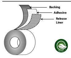
**Backing:** 2 mil Aluminum Foil - Printed
