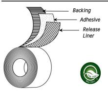
Backing: 2 mil Aluminum Foil - Printed
