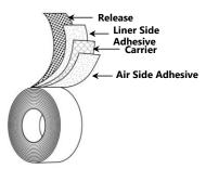
Liner:74# Polycoated KraftLiner Side Adhesive:Acrylic (I632)Backing/Carrier:1 mil PET FilmAir Side Adhesive:Acrylic (I632)
