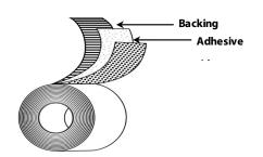
**Backing:** Release Treated PET Film
