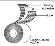
**Backing:** Exterior-Grade Aliphatic Polyurethane
