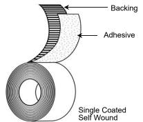
Backing:LDPE FilmAdhesive:AcrylicLiner:N/AColors:Clear, Transparent Orange, White, BlueSpecifications:N/ASize Options:Incremental widths 1/4" - 54" x 108ft
