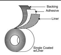
**Backing:** Interior-Grade Aromatic Polyurethane
