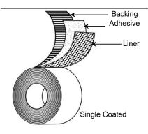
Backing: Low Density Polyethylene
