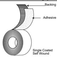
Backing: Release-coated Embossed Polypropylene
