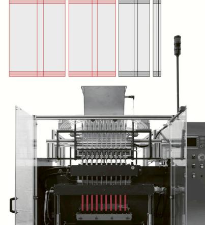
• able to handle reels of up to 900mm width and 1000mm diameter;
