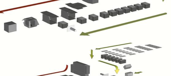
sachet on edge in pre-glued display, inserted with pusher (pushing on side)
