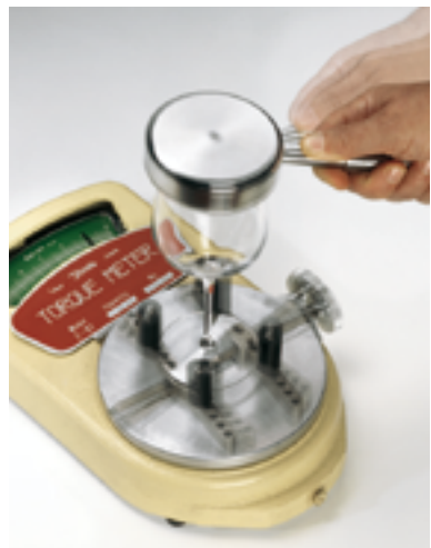
Stem twisting test
